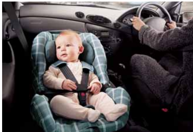
A child in a rear-facing baby seat could be badly hurt by a frontal air-bag if it deployed
